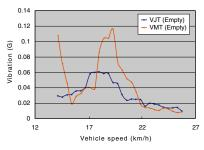
VJT features a lower vibration level than the conventional VMT over a wide vehicle speed range.
